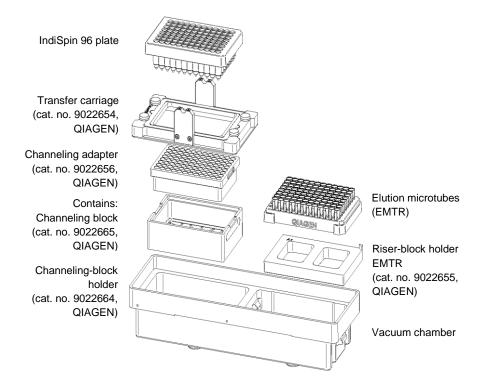
Figure 1: Assembling the vacuum chamber
